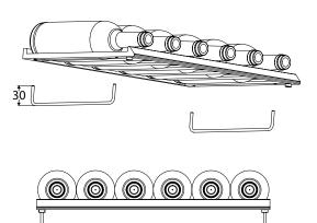
If the height of the storage shelf is to be increased, the set-up device can be attached to the bottom of the shelf. The shelf is subsequently visible when the door is closed. The set-up device is included in the scope of delivery.
